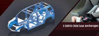
High Tensile Steel Body Construction with Tailor-welded Blanks and Side Anti-intrusion Bars
